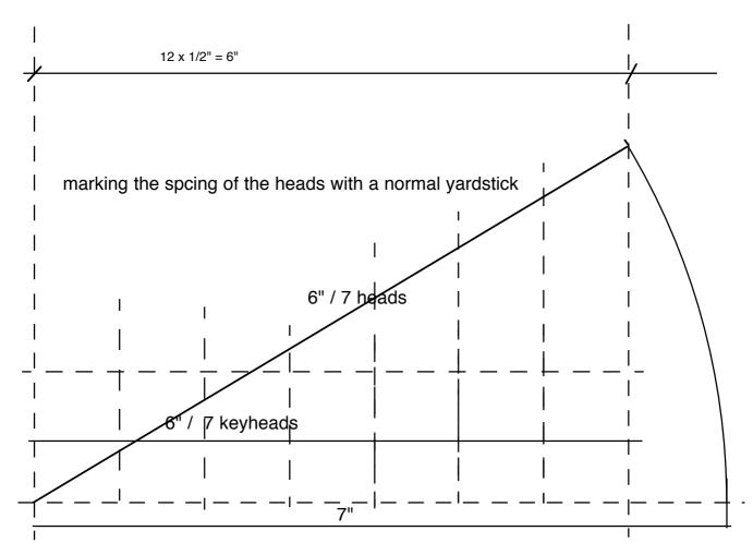
When actually working, the keysheet is covered with n number of individual keyheads to give the correct width prior to any marking out.
