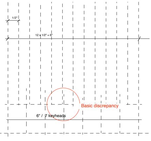
same, too. The remainder is "d" which is wider. In practice as said, the sharps can be marked out with a slotted template (a dedicated square) following the equal "b" -"c" and "e" - "f" simply by using these lines as one edge of the slot; "d" does not of its own get marked out. "G#" is simply centered between the heads "g" and "a", so both "g" and "a" tails don't get marked as such either.
