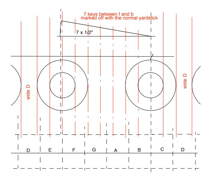
N°. 1 can be applied to Walter: If the octave span at the front is 6", then a naturally wider "d" is the result if the equally wide tails of all notes but "d" were sawn straight back, but the choir centers would not be 1/2", though the octaves would seem to imply this. Turned around: 11x1/2" for "d#" - "c#"; "d" is 7 "= and
